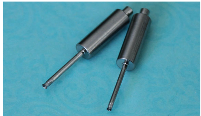
Figure 3. Inserts that are mounted on the rotary tool (UPunch Rotary, Redondo Beach, CA) showing tips of 18-gauge hypodermic needles modified with a flared edge so that the circular cut is directed away from the follicles in order to minimize customary graft damage.
